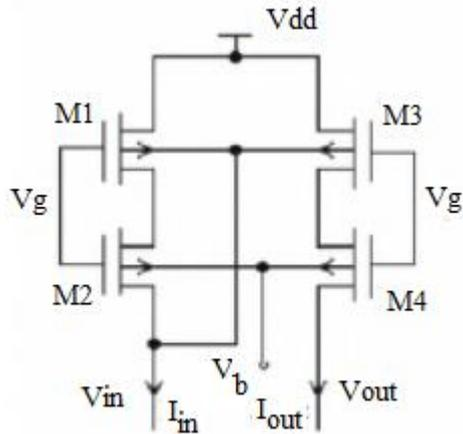
Fig.8 PMOS bulk-driven cascade current mirror
