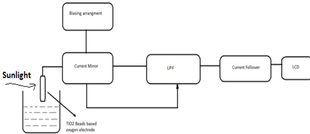
Fig. 4 Block diagram of proposed scheme
