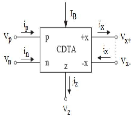
Fig. 2 : Electrical symbol of CDTA
