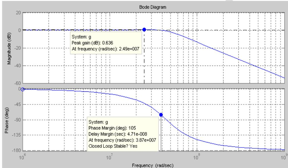
Fig.6 bode plot of the above transfer function
