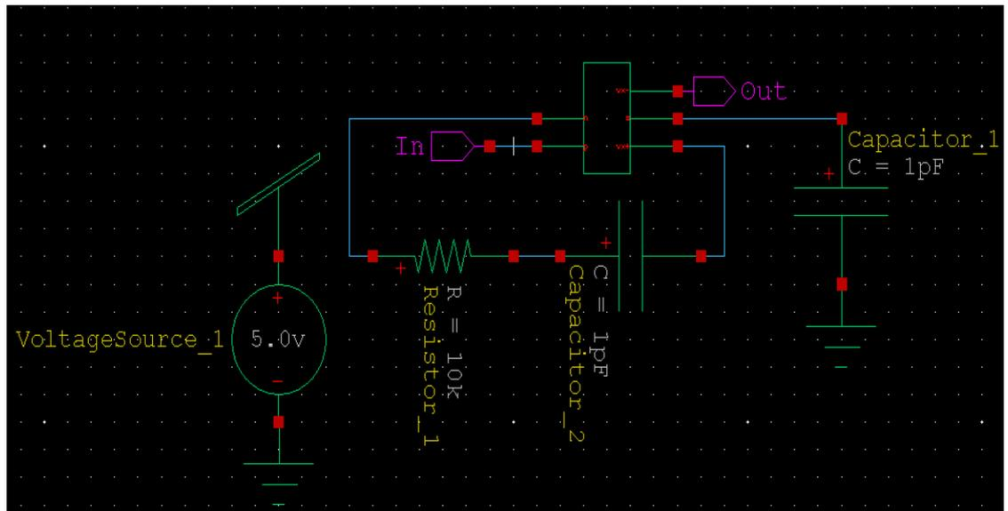
Fig.9 Circuit diagram of proposed scheme
