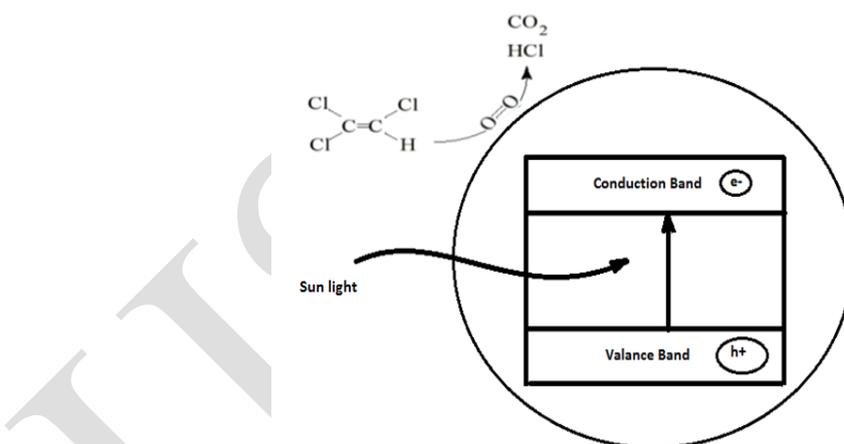
Fig.1: Diagram to show Photocatalysis
