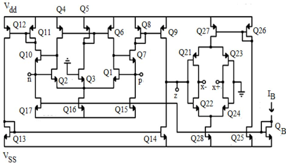
Fig. 3: Circuit diagram of CMOS based CDTA
